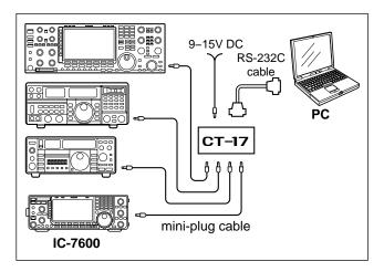
When the transceiver is connected to a PC with the USB cable (third party), the optional CT-17 is not required.
