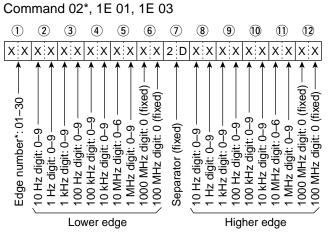
\* Edge number setting is not necessary with command 02.
