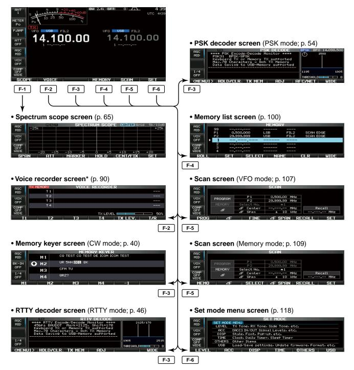
\*Previously selected screen, TX or RX memory, is displayed. Push **[T/R] (F-6)** to switch the screen.
