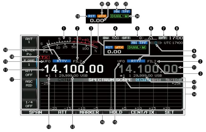
S/RF METER (pgs. 35, 126) Shows the signal strength while receiving. Shows the relative output power, SWR, ALC, VD, ID or compression levels while transmitting.
