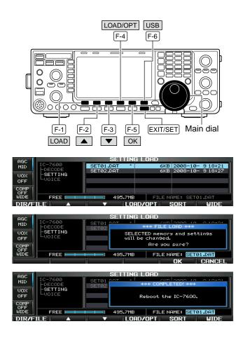
By loading the saved setting file from the USB-Memory, you can easily set up another IC-7600 or apply the several operators settings to one IC-7600.
