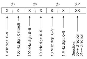
\*No need to enter for transverter offset frequency setting. <sup>†</sup>Transverter offset only; Fix to '0' for split offset setting.
