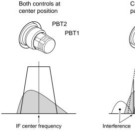
Cutting the lower Cutting both lower and passband edge PBT2 PBT1 Passband
