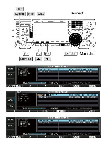
When a PC keyboard is connected to [USB] connector on the front panel, the file name can also be edited from the keyboard. In this case, a USB hub is required. The file name, saved in the USB-Memory, can be renamed from the transceiver as desired.
