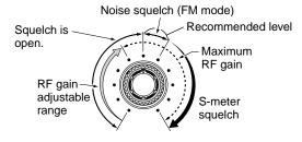
• When functioning as RF gain control (Squelch is fixed open; SSB, CW, RTTY, PSK only)
