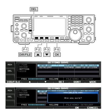
**RECOMMENDATION!** Deleting the setting file is irreversible. Confirm the contents before deleting a setting file!
